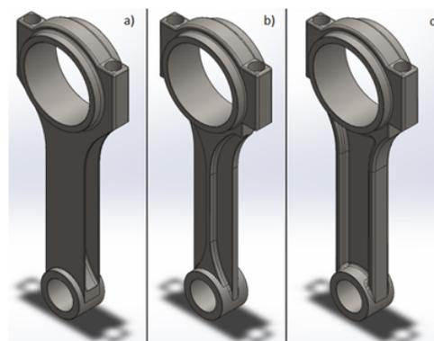
Fig. 2. Connecting rod models manufactured. a) genuine model, b) model with a side notches of the shank, c) model with a notch in the middle of the shank.
