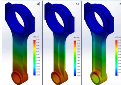
Fig. 5. Displacements - isometric view. a) genuine model, b) model with a side notches of the shank, c) model with a notch in the middle of the shank
