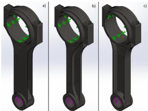
Fig. 3. The analysed model with generated mesh and the boundary conditions a) genuine model, b) model with a side notches of the shank, c) model with a notch in the middle of the shank
