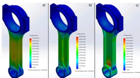
Fig. 4. Stress distribution-isometric view. a) genuine model, b) model with a side notches of the shank, c) model with a notch in the middle of the shank
